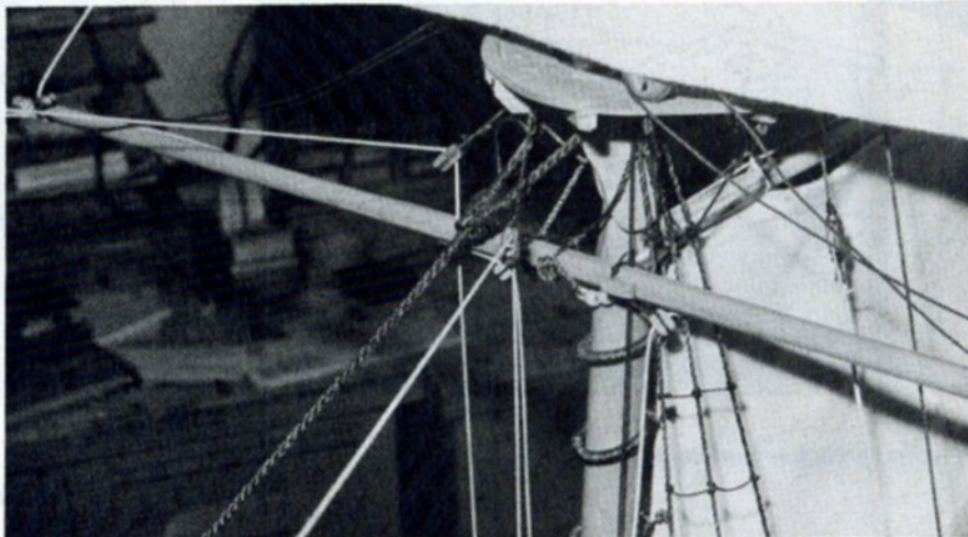
BLOCKS ON MIZZEN mast that operate the main yard.
