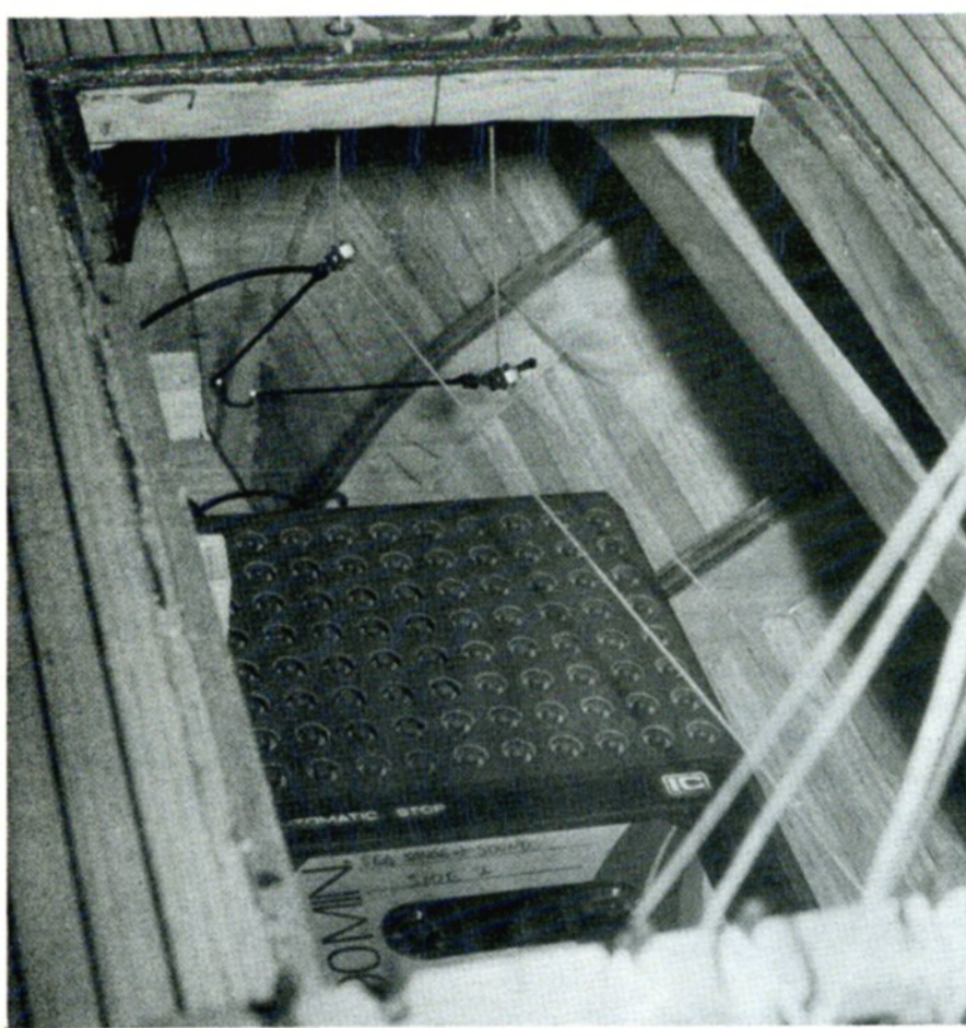
BLOCKS AND PULLEYS with elastic take the slack when the sail winch is operated. The tape player for sound effects can be seen at the bottom.
