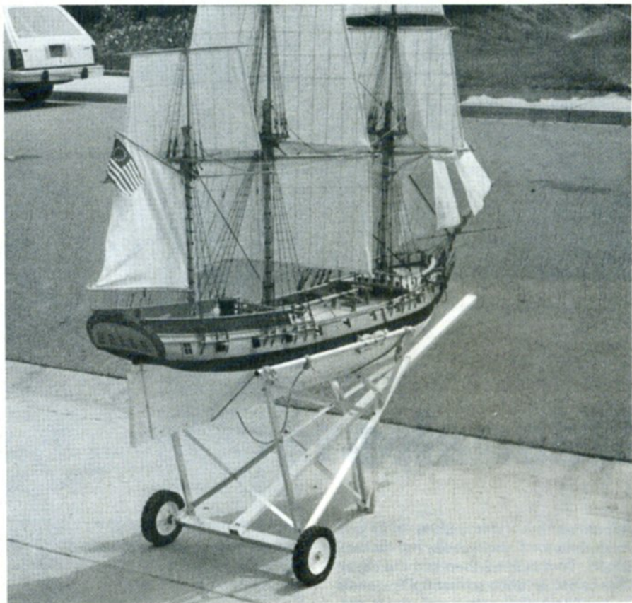
AN ALUMINUM custom built carriage was made to move and launch the ship without strenuous effort.
